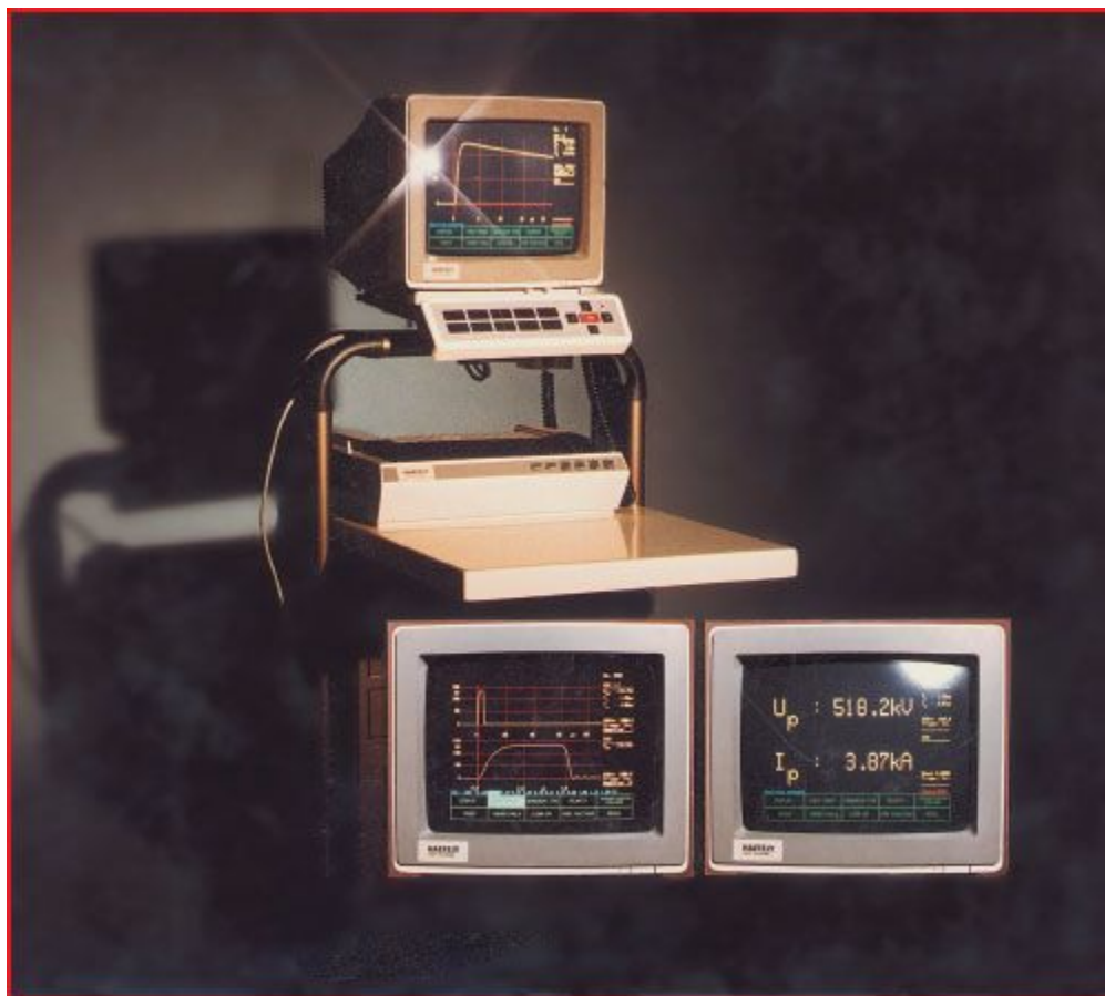
Digital Impulse Analysis System (DIAS) for Impulse Voltage and Current Measurement System. (Courtesy: Haefely Trench)
