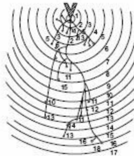
Fig. 4.2 Breakdown channels in perspex between point-plane electrodes. Radius of point 0.01 in, thickness 0.19 in. Total number of impulses 190. Number of channels produced 16; (n) point indicates end of nth channel. Radii of arcs increase in units of 10^{-2} in.
