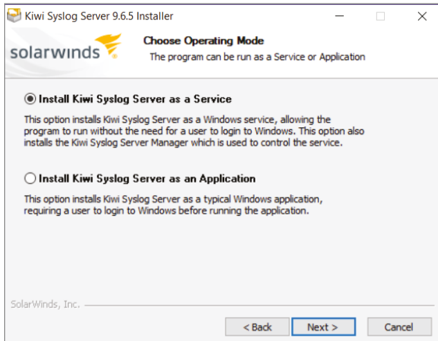
Figure 9.10: Choosing a service or application operating mode with Kiwi Syslog Server
